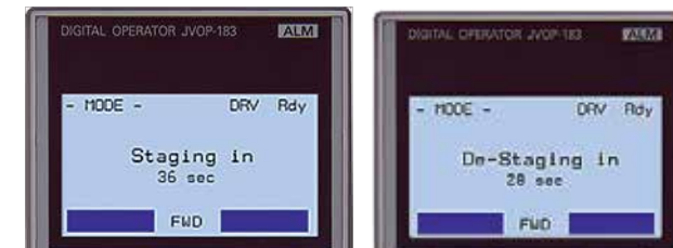
Typical Multiplex Keypad Messages
