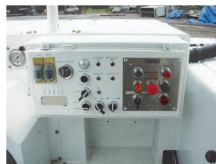
Operator Station installed
