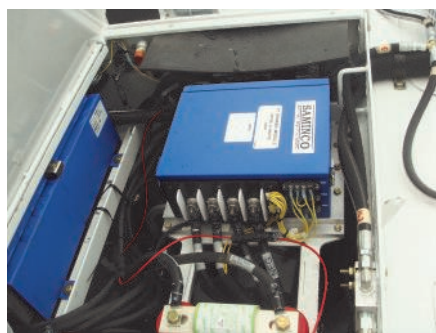
Brake Module installed
