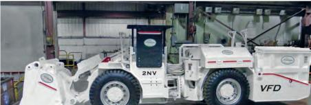
Before and After - images of an LHD rebuild where electric drives and battery electric specialist Saminco converted the machine from diesel to battery power for the lead rebuilder, client Highland Machinery
