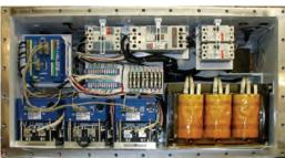
Three drive system for shuttle cars
