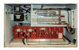
Q750 system mounted in explosion proof box with swinging panel closed.
